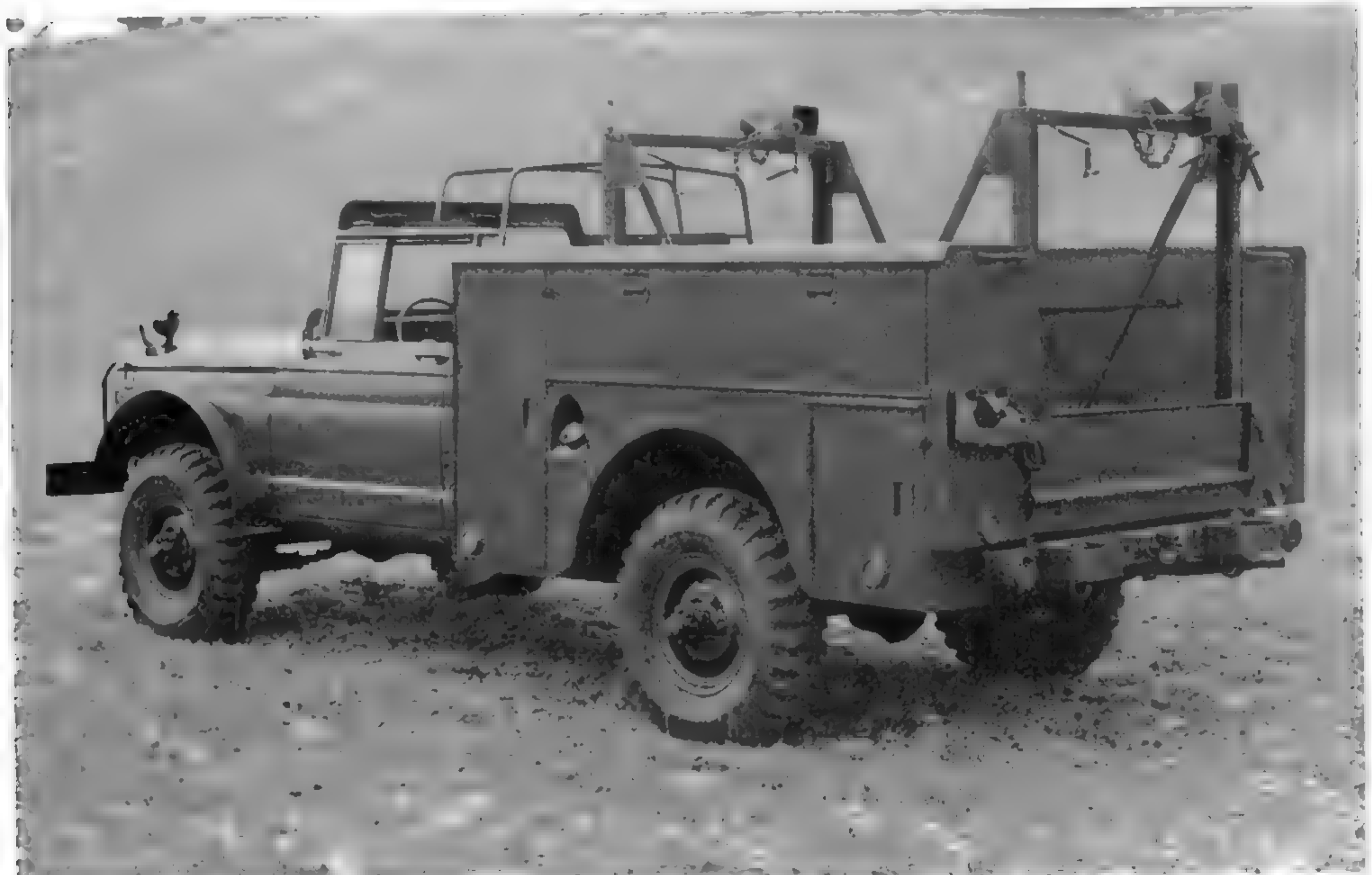
This is the XM726 1 1/4-ton telephone maintenance truck. Its bed is much different than the 6217 bed, but very similar to the bed of the G-741-based V-41/GT. (U.S. Army photo)
